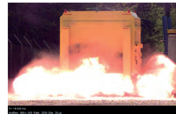
Blast test in an underbelly threat scenario with home-made explosives
