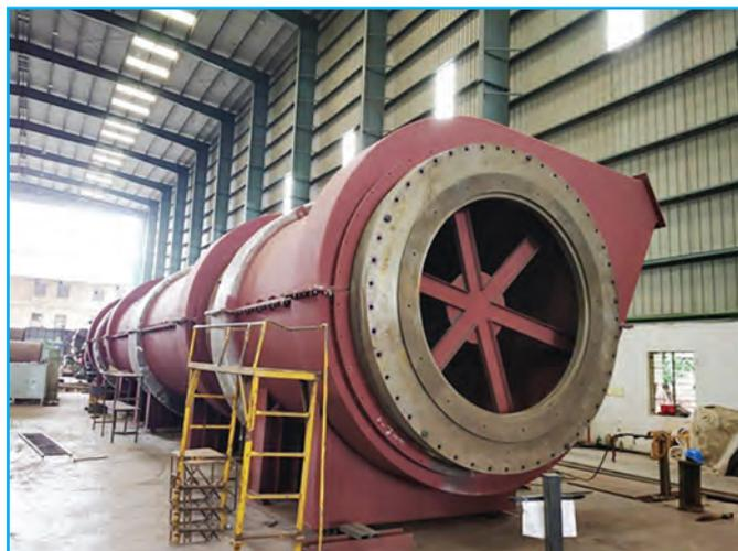
HF Kiln with Heating Jacket for M/s. TANFAC Industries Ltd. ready for dispatch
