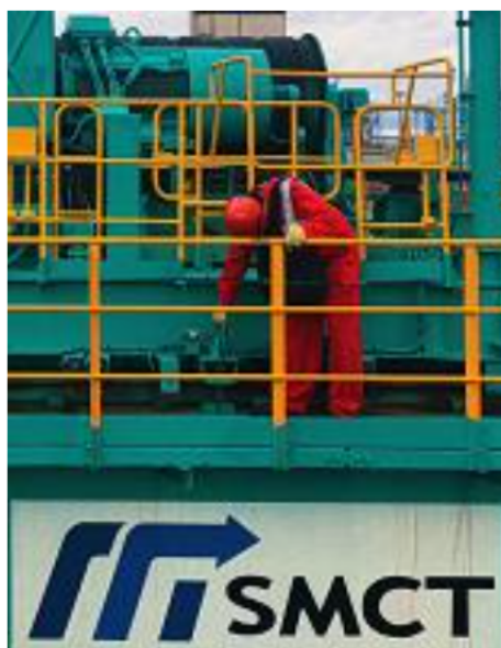
▲SMCT-removing anchoring device after typhoon left
