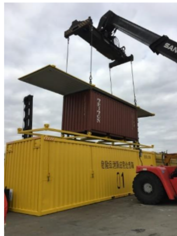
(Box for Leaky Dangerous Goods)
