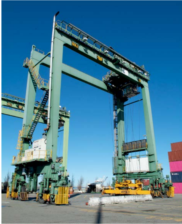
One of 13 retrofitted battery-powered hybrid gantry cranes.
