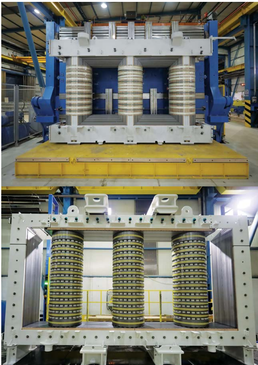
Power transformer core and shunt reactor core
