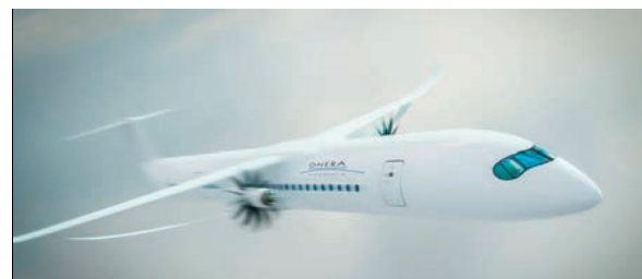
Innovations in the AWATAR project: shrouded wings, laminar wings and open-fan engines.
