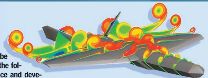
Mach number field around an example of a configuration studied as part of the COBRA ARF, using RANS calculations carried out with SoNICS
