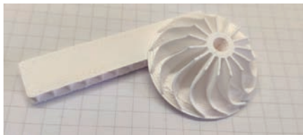
Alumina part obtained by FDM: a turbine part and a honeycomb sandwich panel (grid: 5x5 mm).
