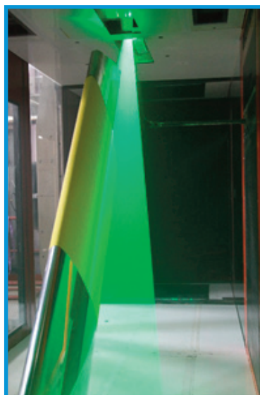
Experimental set-up and laser plan for PIV measurements.
