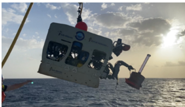
Instrument to measure the vertical velocity of the diffuse flow of hydrothermal vents.
