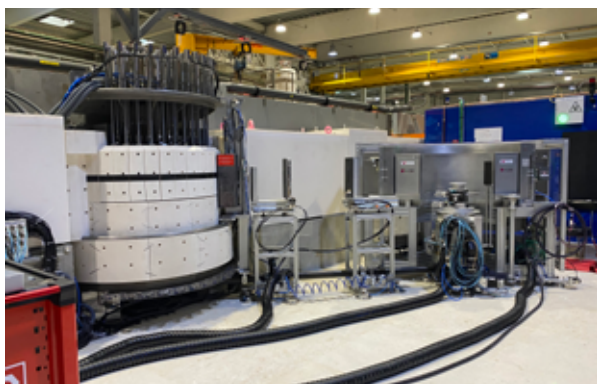
View of XtremeD in December 2022, with all components installed and in the process of wiring and alignment (without neutrons).
