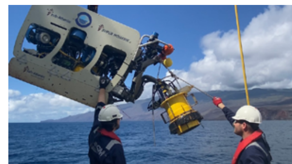
Sensor-bearing hood for monitoring diffuse hydrothermal fluid outflows.
